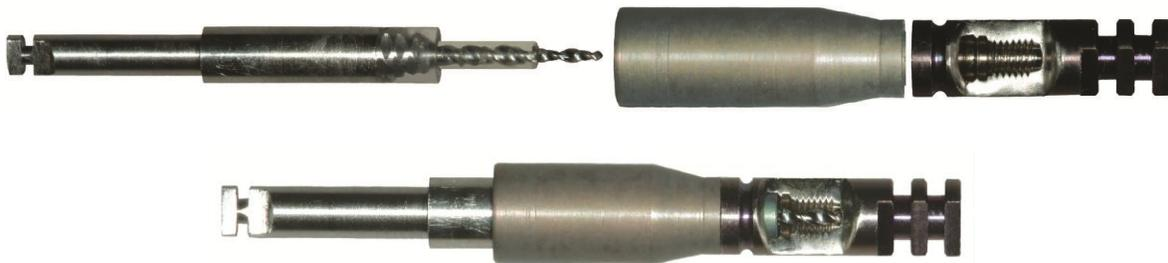
4. Modified drill prototype, guide and windowed analog both separate and assembled.
